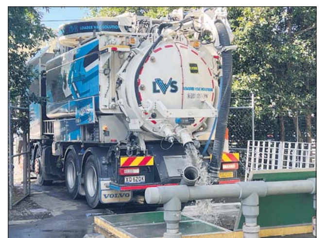
A truck dumps sewage into a pumping station in Byron. Photo Jeff Dawson
