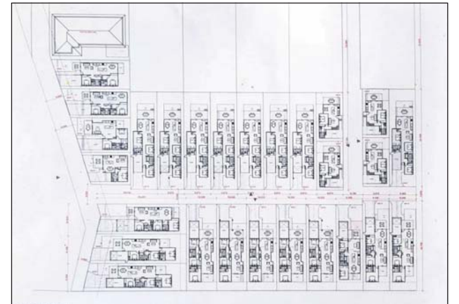
An internal, one-way, loop driveway is proposed, 'with a maximum width of 6.7m to allow for garbage collection and emergency vehicle access'. Image from proposal
